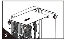
Unscrew the 3 screws of "a" positions, then push the top glass backward according to the arrow direction to disassemble it.
