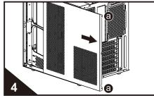
Unscrew the screw of "a" position then slide out right side panel backward to disassemble it.
