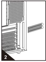
Break off PCI slot covers of the corresponding positions.
