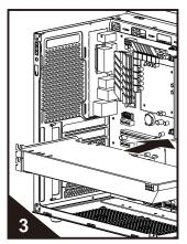
Insert VGA card into the slot of M/B according to the arrow direction;
