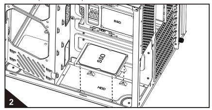
Put 2.5"SSD\*1 on the bottom panel, align screw holes then fix it by screws from the bottom.
