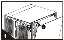
Unscrew the screw on rear panel which secured left glass, push the left glass outward according to the arrow direction as shown in the illustration to disassemble it.
