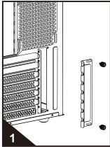
Unscrew the screws of the fastening bar of the PCI slot covers, remove the fastening bar.
