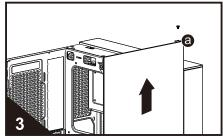
Unscrew the screw of "a" position, then take the front glass upward according to arrow direction to disassemble it.
